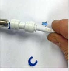
Pull the hose back out of the white collet to lock it into place.
